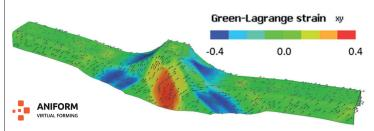
increases the design flexibility. Wrinkle formation depends upon the fine balance of the composite's resistance to shear, slip and bending deformations. Therefore, accurate modeling of these mechanisms is essential. (See section "How it works" for more background information.)
